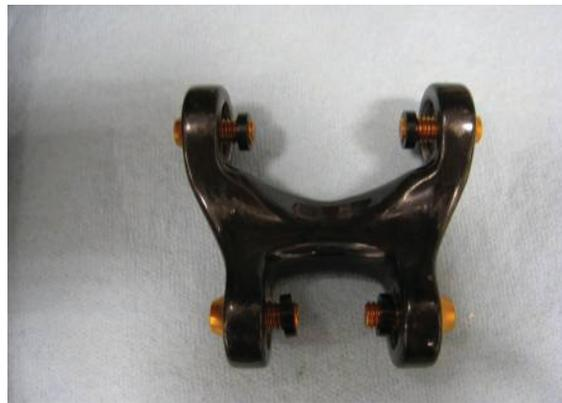
Install rocker bolts using grease or anti-seize. Torque to (10 lb.ft, 120 lb.in, 13 Nm.)
