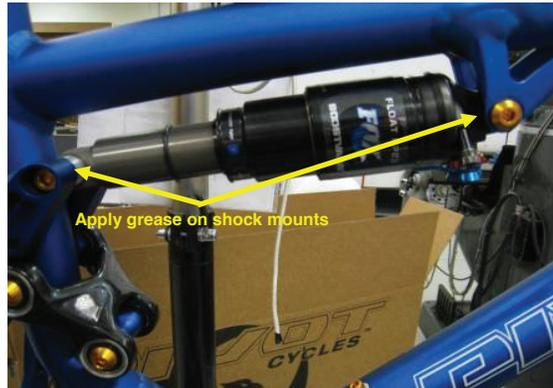
Install long shock bolt using anti-seize and torque to (10lb. ft, 120lb. in, 13Nm.)
