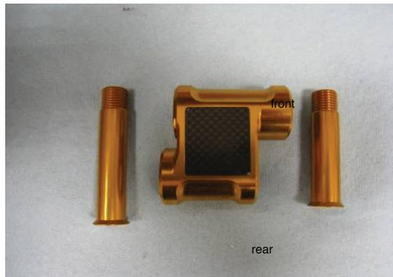
Use anti-seize and torque link pins to ( 27lb ft, 35 Nm. )
