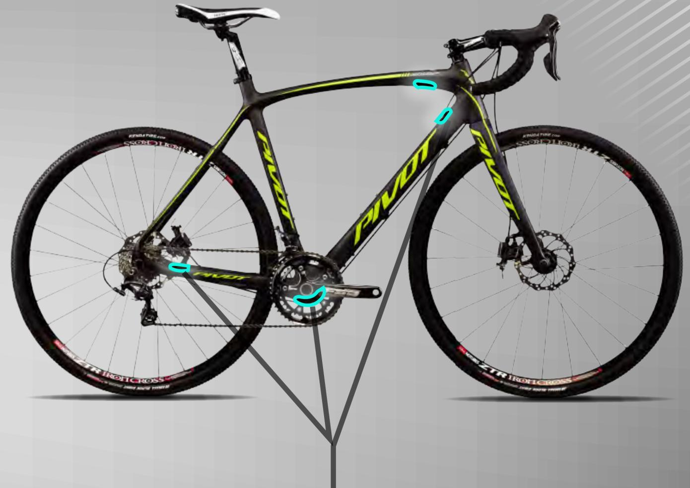
**Internal cable routing** adapts easily to either electronic or cable actuated shift systems. While the stealthy internal top tube brake routing can be totally disguised in disc brake form or cleanly hidden out of the way with cantilever brakes making **portaging your bike a clean, snag free affair.**
