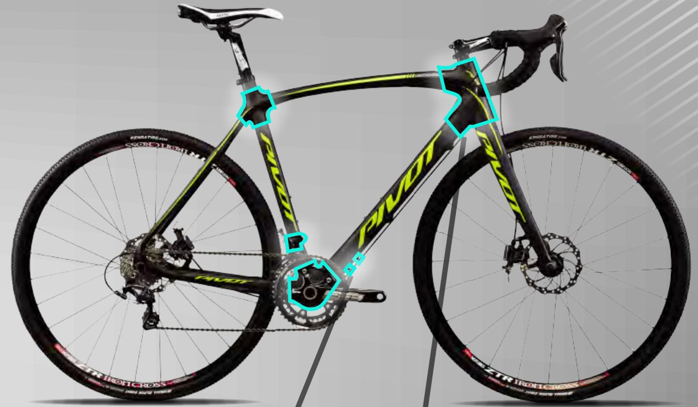
Designed to be **Di2 compatible** with internal wire routing ports and battery specific downtube mounts
