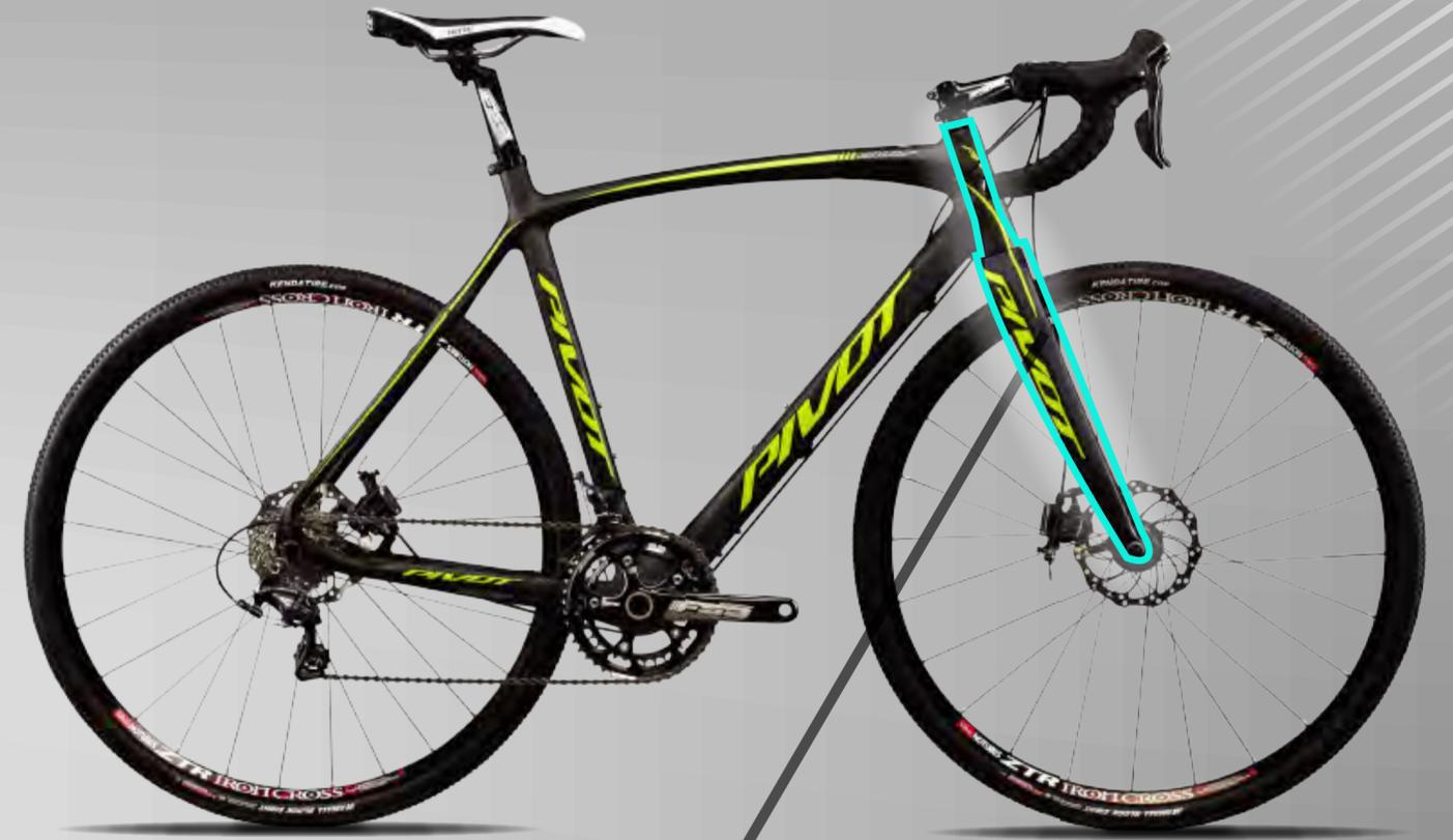
The Vault's 1.5 inch tapered steerer fork with oversize crown optimizes stiffness, increases steering precision, provides great mud clearance while eliminating brake chatter
